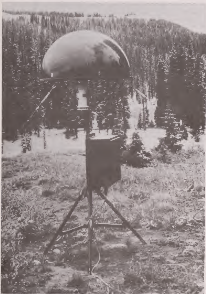
Data collection platform and transmitter used by Project Skywater in connection with the Earth Resources Technology Satellite (ERTS). (Courtesy of the Bureau of Reclamation.)
