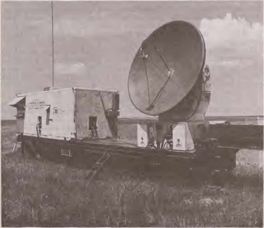
NOAA 1 X-band Doppler radar operated by the Wave Propagation Laboratory of the National Oceanic and Atmospheric Administration. (Courtesy of the U.S. Department of Commerce.)
