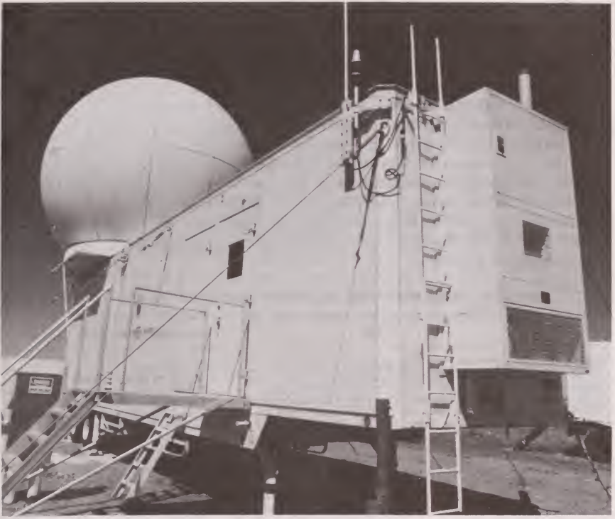
Portable radar used in Project Skywater. (Courtesy of the Bureau of Reclamation.)
