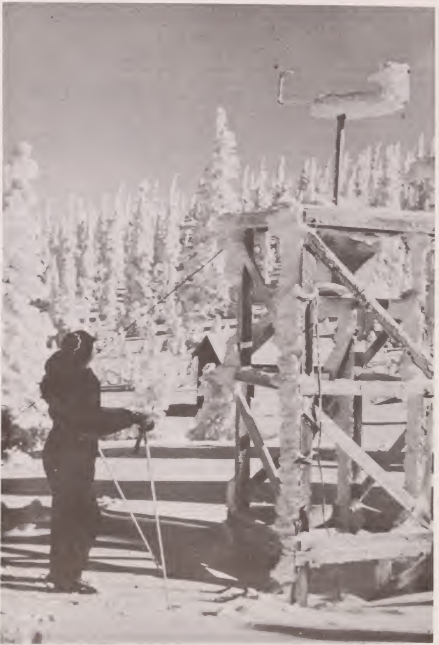
Rime ice conditions at sensing device which measures intensity of snowfall. (Courtesy of the Bureau of Reclamation.)
