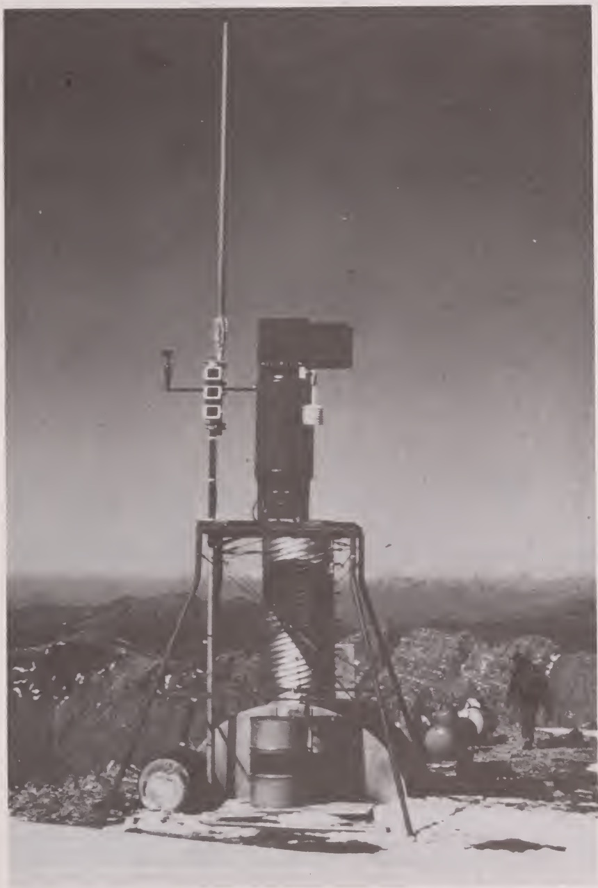
Remotely operated cloud seeding generator similar to those used in the Colorado River Basin Pilot Project. (Courtesy of the Bureau of Reclamation.)
