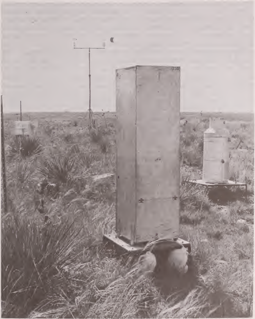
Precipitation instrument site, including, from left to right, hailcube, anemometer, rain/hail separator, and Belfort weighing precipitation gage. (Courtesy of the National Science Foundation.)
