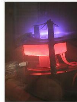
DC plasma (violet) enhances the growth of carbon nanotubes in this laboratory-scale PECVD apparatus.
